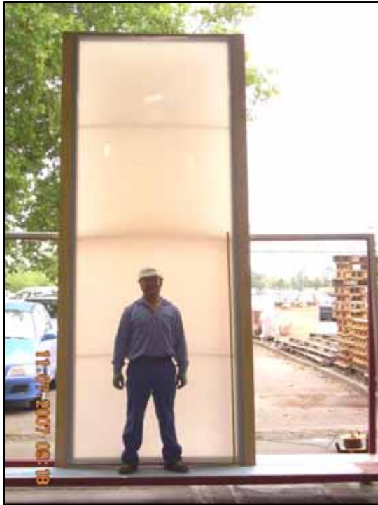
Project in the US with translucent Aerogel-filled ETFE-Roof-Panels, U-Value < 0,25 W/m 2 K
